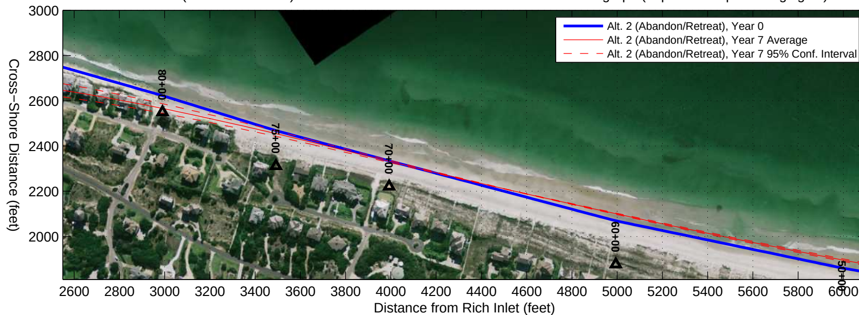
Alternative 2 (Abandon/Retreat) GENESIS Results with October 2007 Aerial Photograph ( http://earthexplorer.usgs.gov/ )
