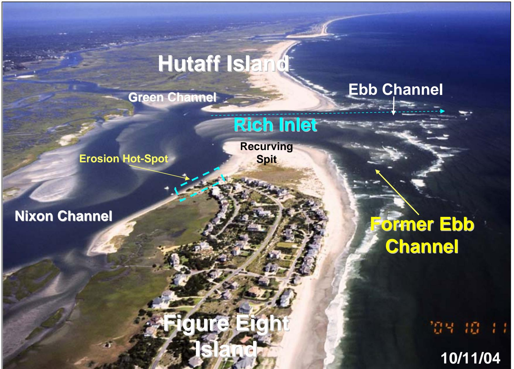
**Figure 34.** Oblique aerial photograph (10/11/04) illustrating the oceanfront conditions along northern end of F8I, the interior channels and location of the estuarine erosion hot-spot (light blue dashed line box).
