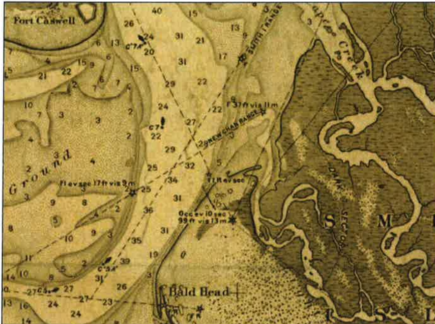
Figure 12. 1923 C&GS chart showing realignment of the Bald Head Channel reach beacon, installation of a front beacon for the Smith Island Channel reach and a front-range beacon for the Southport Channel reach.
