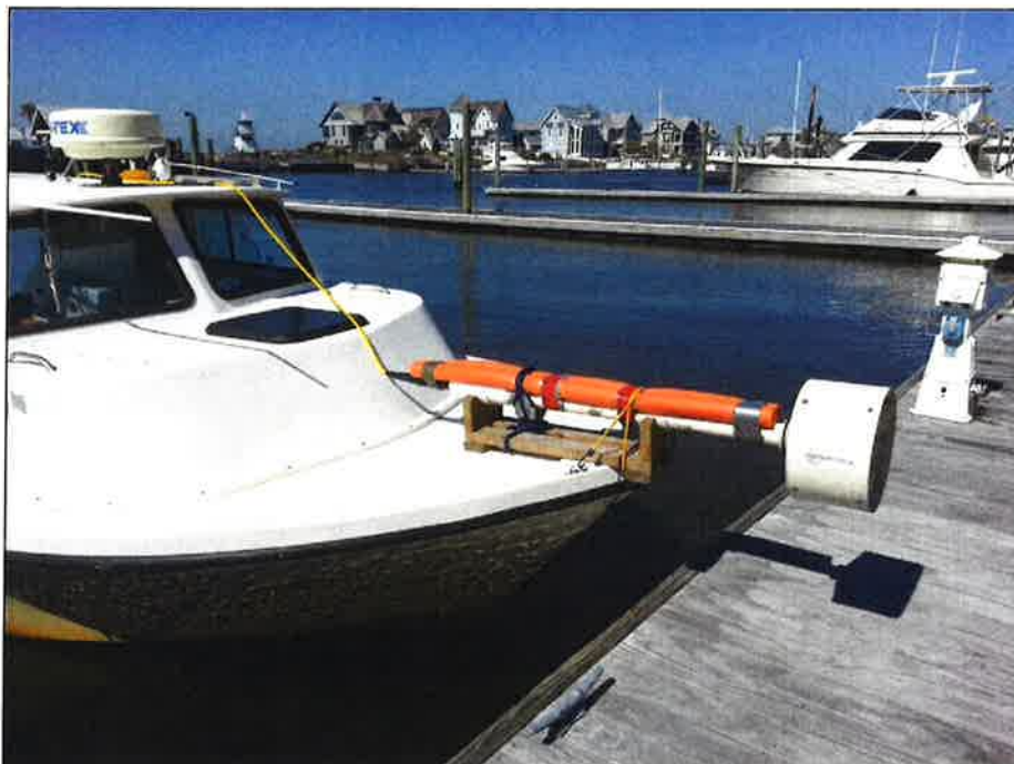
Figure 4. Bow mounting the GEOMETRICS G-881 cesium vapor magnetometer.
