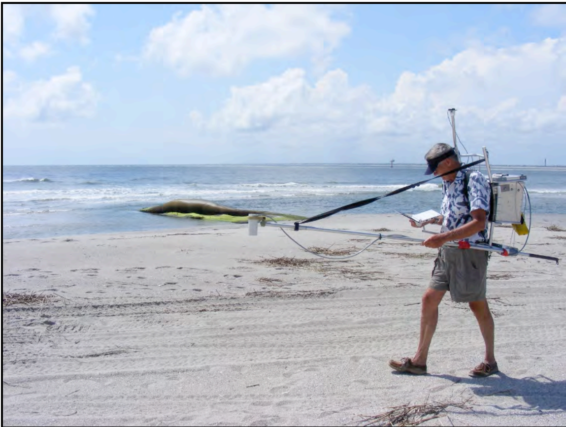
Figure 2. The G-856 magnetometer, Trimble DGPS and PC used for the terrestrial remote sensing survey.
