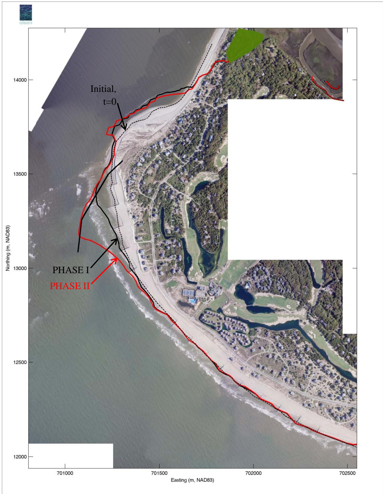
Figure 11: Comparison of MLLW predicted shoreline contours at year 9 for the Phase I and Phase II terminal groin scenarios.
