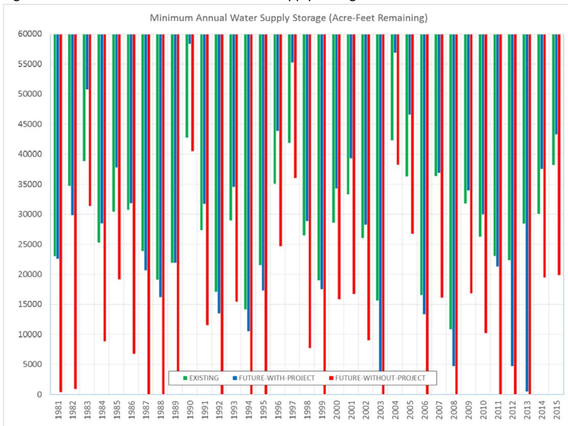
Figure 10. Falls Lake Water Supply Storage Duration for All Model Conditions
