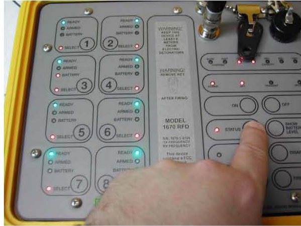
Figure 4-13 Manually checking STATUS
