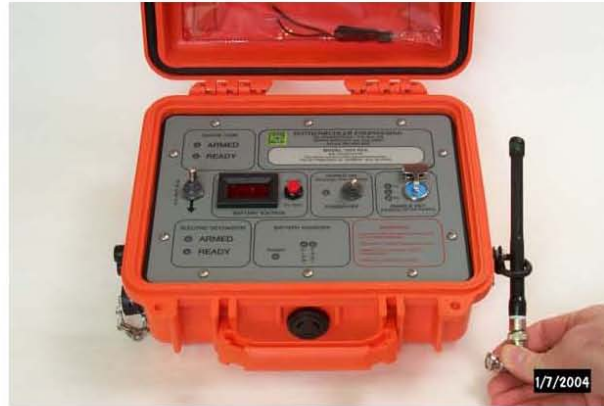
Figure 4-2 Remote Antenna Installation
