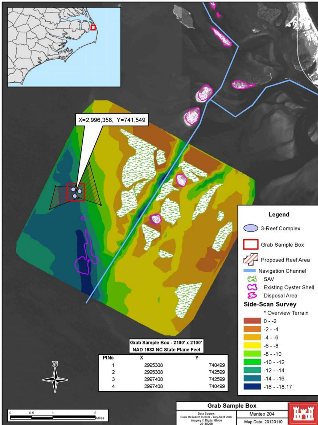
Figure 1: Location of proposed dredge disposal site west of the navigation channel. Inset shows a close-up of the proposed dredge site, with preliminary sample locations shown in red.
