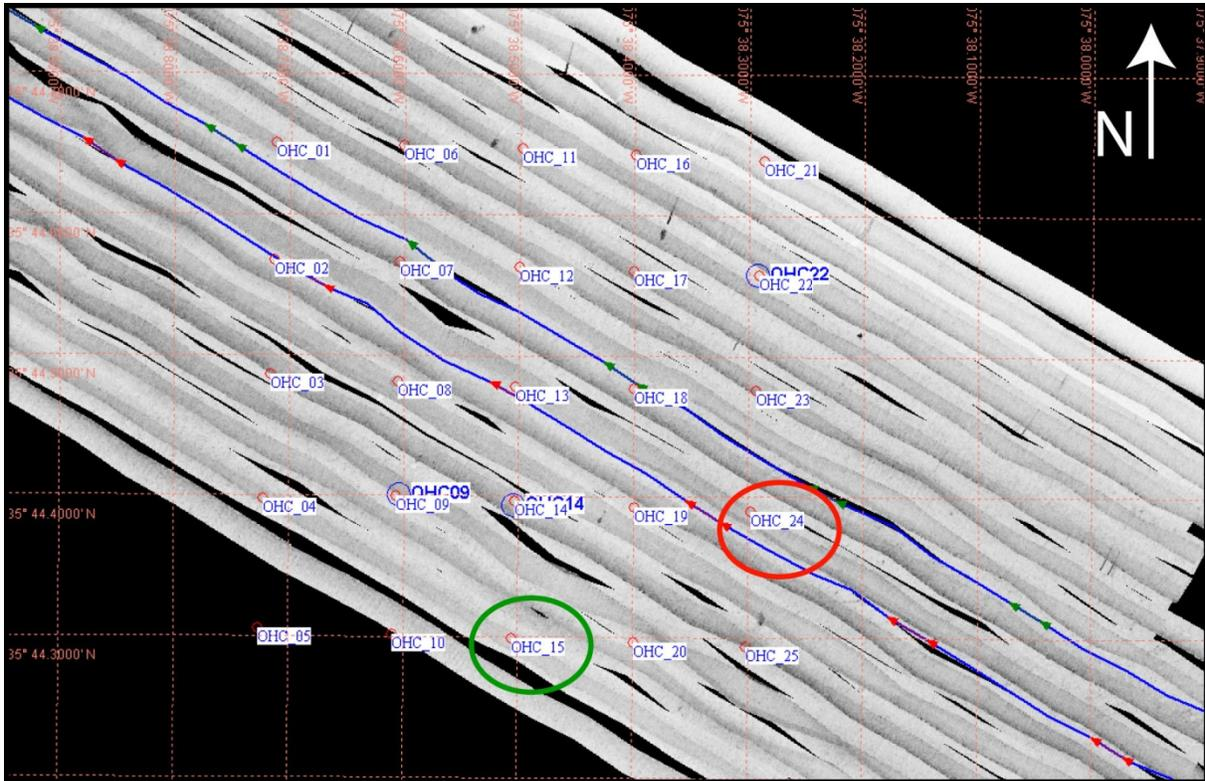
**Figure 9: Reprocessed sidescan sonar data. Red circle indicates a sandy sample (OHC 24: 93.87% sand); green circle indicates a muddy sample (OHC 15: 67.91% sand).**
