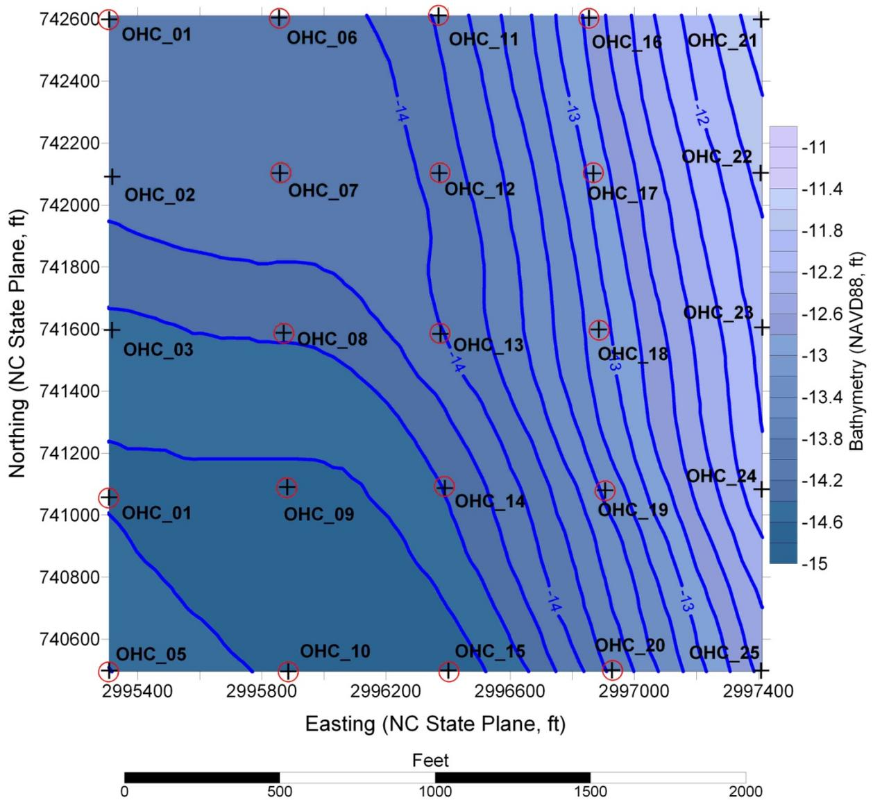
Figure 2: Bathymetry of the proposed dredge site. Grab sample locations are indicated by black crosses. Red circles indicate the presence of various polychaetes in the sediment samples.
