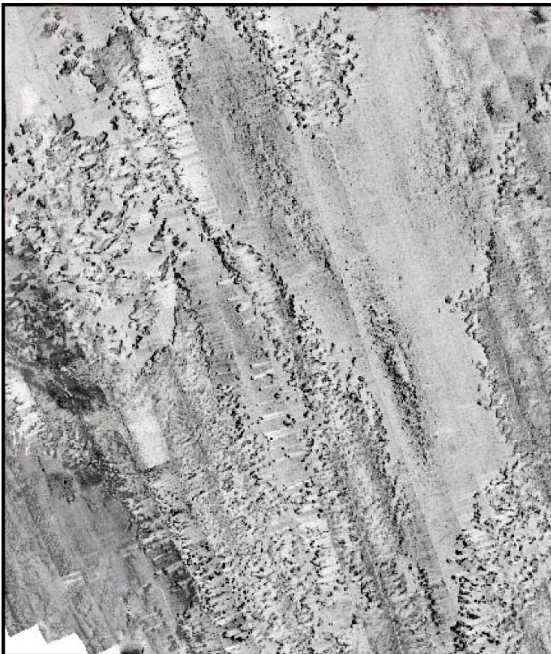
**Figure 3. Processed side-scan mosaic of multiple survey lines showing areas of SAV (darker rough areas) and fine sand (light colored smooth areas)**
