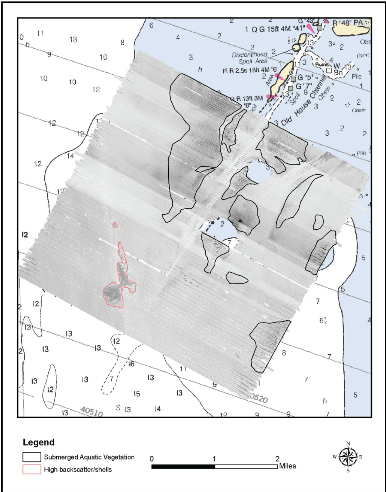
Figure 5. Old House Channel Side-Scan mosaic with areas of SAV and high backscatter identified by polygons
