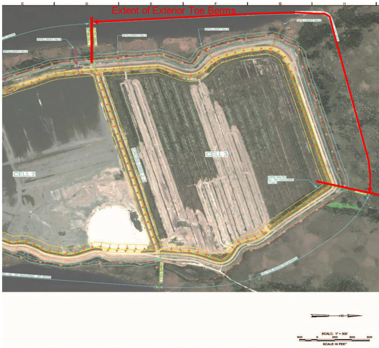
Figure 1. Extent of Exterior Toe Berms around Cell 3.
