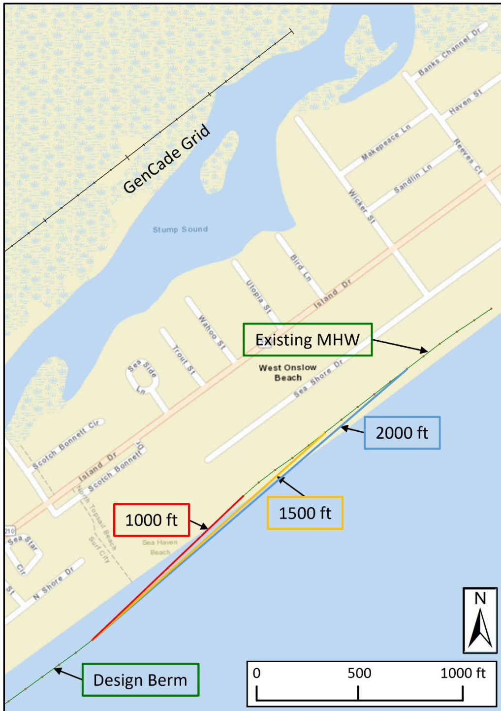
Figure 4. FWP Transition design MHW contours – northeast shoreline.
