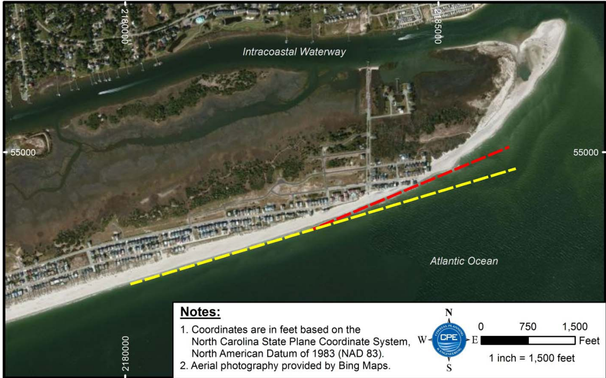
Figure 9. East end of Ocean Isle Beach showing change in shoreline orientation.
