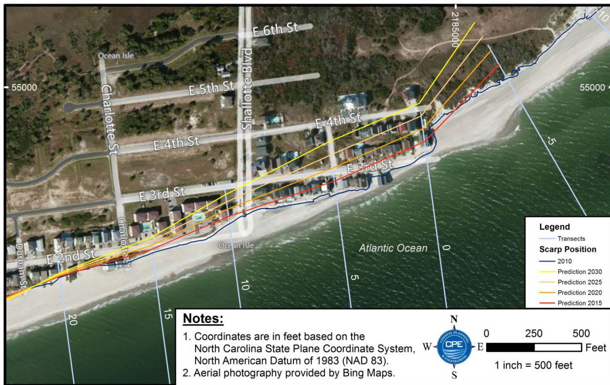
Figure 4. Predicted scarp positions on east end of Ocean Isle Beach in 2015, 2020, 2025, and 2030 based on erosion rates at each station.
