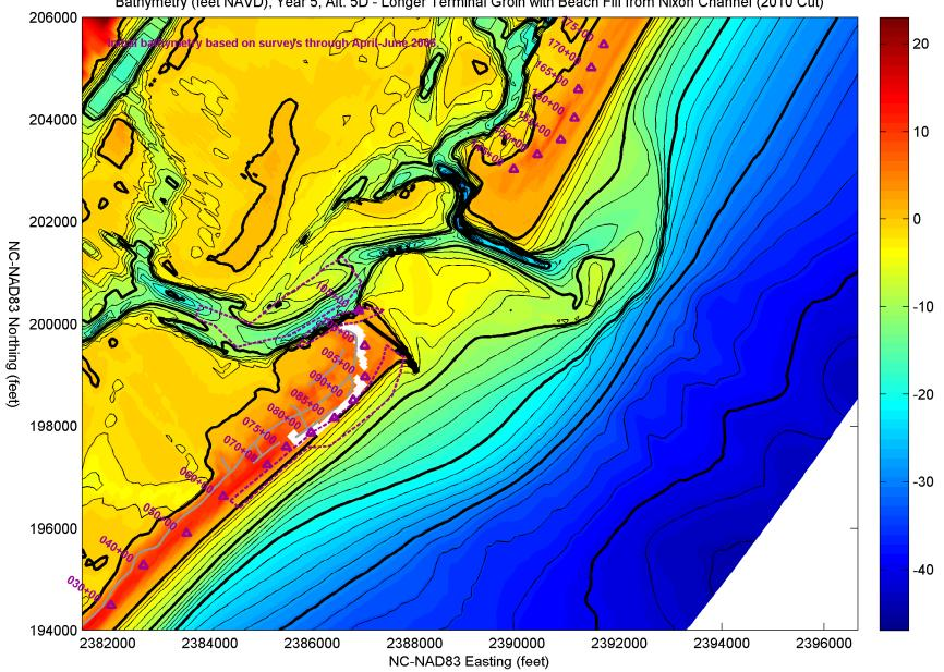
Bathymetry (feet NAVD), Year 5, Alt. 5D - Longer Terminal Groin with Beach Fill from Nixon Channel (2010 Cut)
