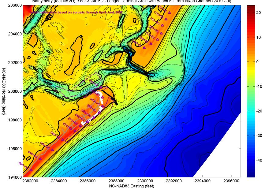
Bathymetry (feet NAVD), Year 3, Alt. 5D - Longer Terminal Groin with Beach Fill from Nixon Channel (2010 Cut)
