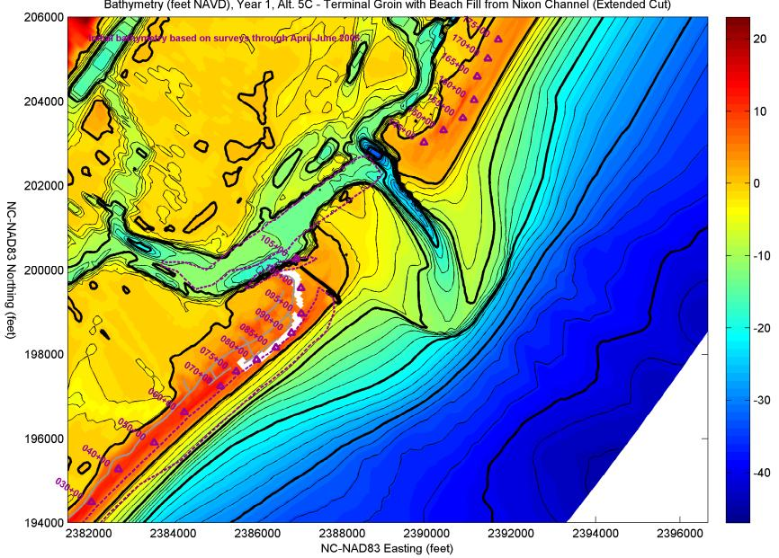
Bathymetry (feet NAVD), Year 1, Alt. 5C - Terminal Groin with Beach Fill from Nixon Channel (Extended Cut)
