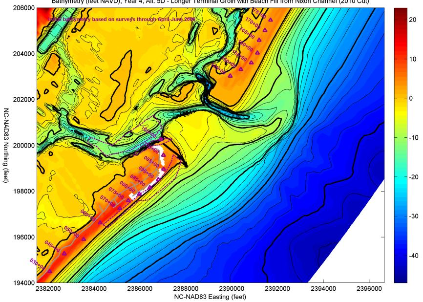
Bathymetry (feet NAVD), Year 4, Alt. 5D - Longer Terminal Groin with Beach Fill from Nixon Channel (2010 Cut)
