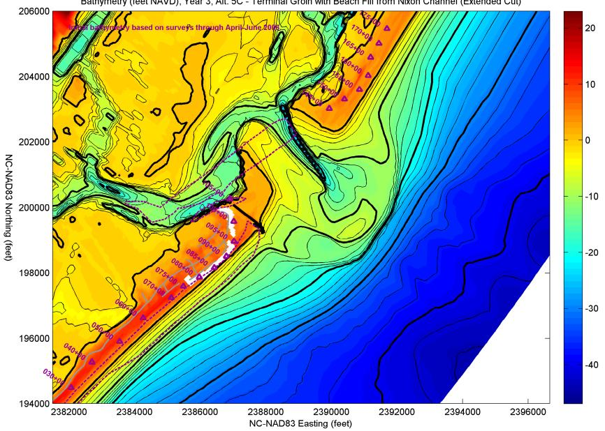
Bathymetry (feet NAVD), Year 3, Alt. 5C - Terminal Groin with Beach Fill from Nixon Channel (Extended Cut)
