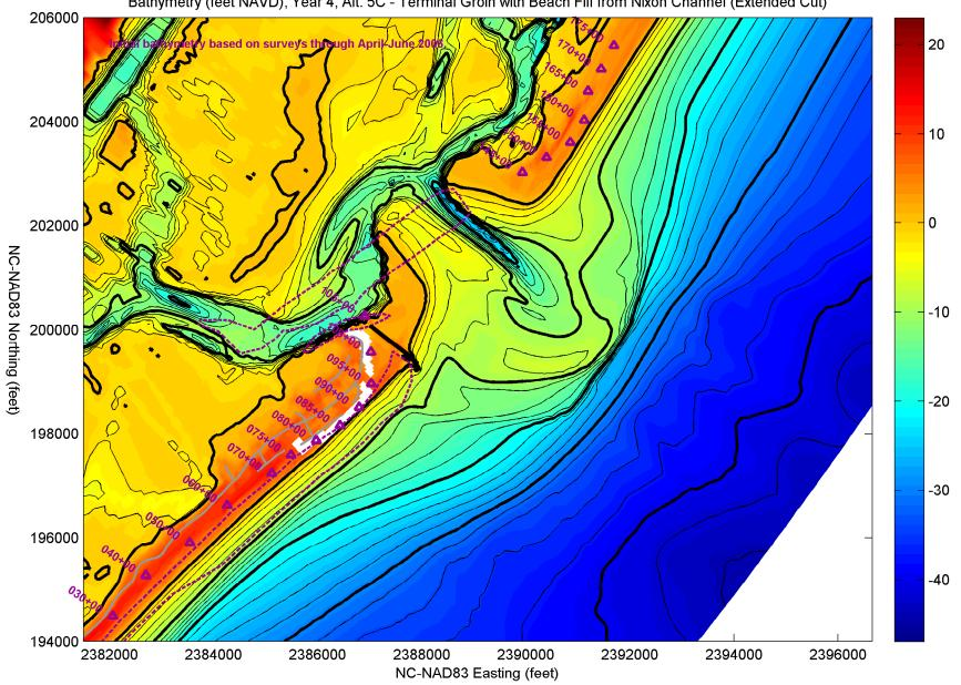
Bathymetry (feet NAVD), Year 4, Alt. 5C - Terminal Groin with Beach Fill from Nixon Channel (Extended Cut)
