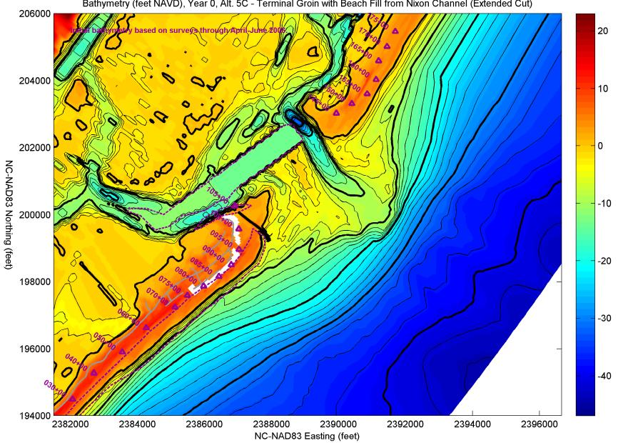
Bathymetry (feet NAVD), Year 0, Alt. 5C - Terminal Groin with Beach Fill from Nixon Channel (Extended Cut)
