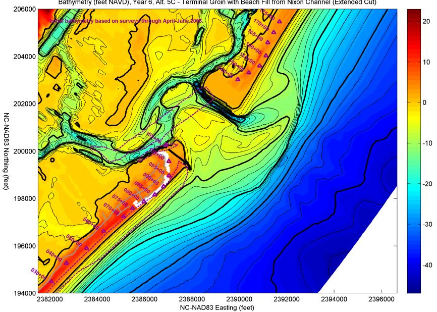
Bathymetry (feet NAVD), Year 6, Alt. 5C - Terminal Groin with Beach Fill from Nixon Channel (Extended Cut)
