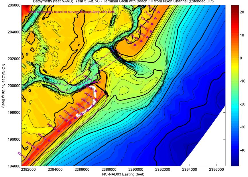
Bathymetry (feet NAVD), Year 5, Alt. 5C - Terminal Groin with Beach Fill from Nixon Channel (Extended Cut)
