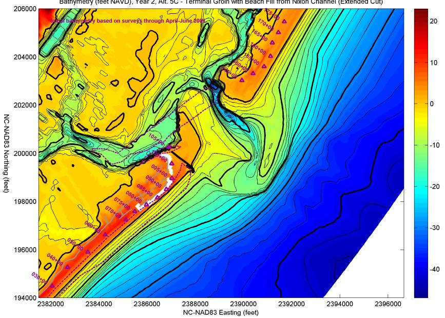
Bathymetry (feet NAVD), Year 2, Alt. 5C - Terminal Groin with Beach Fill from Nixon Channel (Extended Cut)
