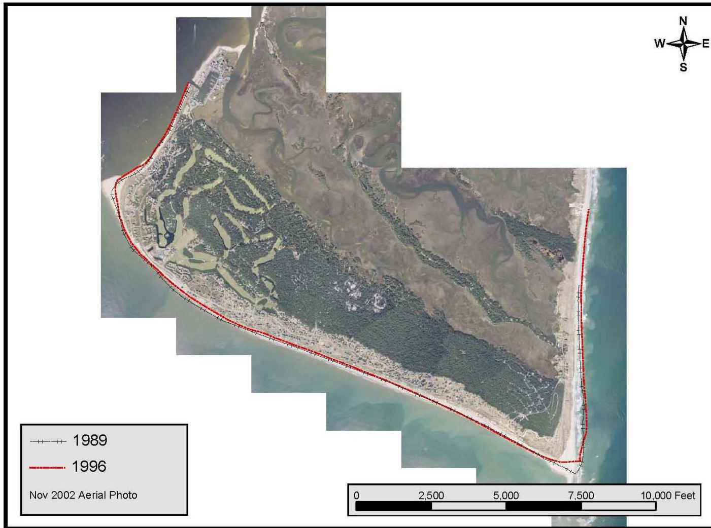
Figure 4.6. Bald Head Island Shoreline Positions (1989 and 1996) (Source: USACE Wilmington Harbor Monitoring Report No. 1 – 2004)
