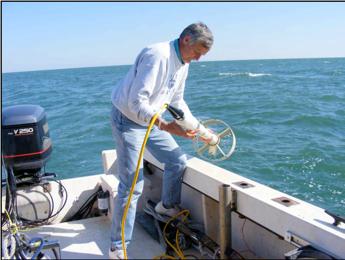
Figure 2. Launching the EG&G GEOMETRICS G-881 magnetometer.
