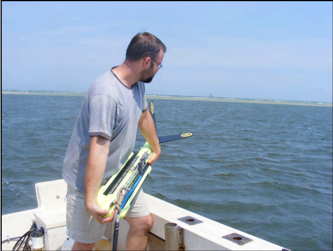
Figure 3. Launching the KLEIN SYSTEM 3900 digital sidescan sonar.
