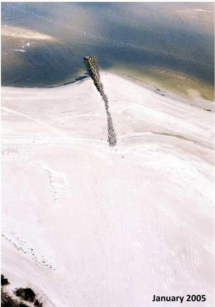
Figure x.x: Chronology of South Amelia Island Leaky Terminal Structure constructed at Amelia Island State Park, Nassau County, Florida.
