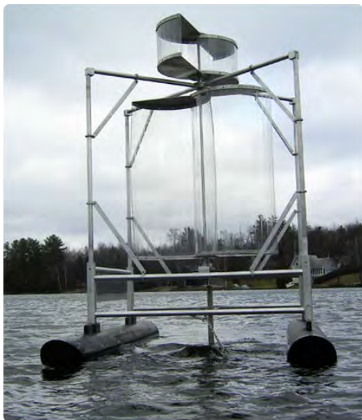
Figure 7 - Example of Wind Powered In-Lake Long-Distance Circulator
