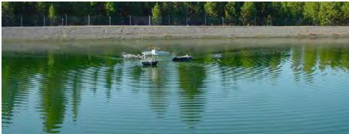
Figure 30 - Image of Circulator in Operation
