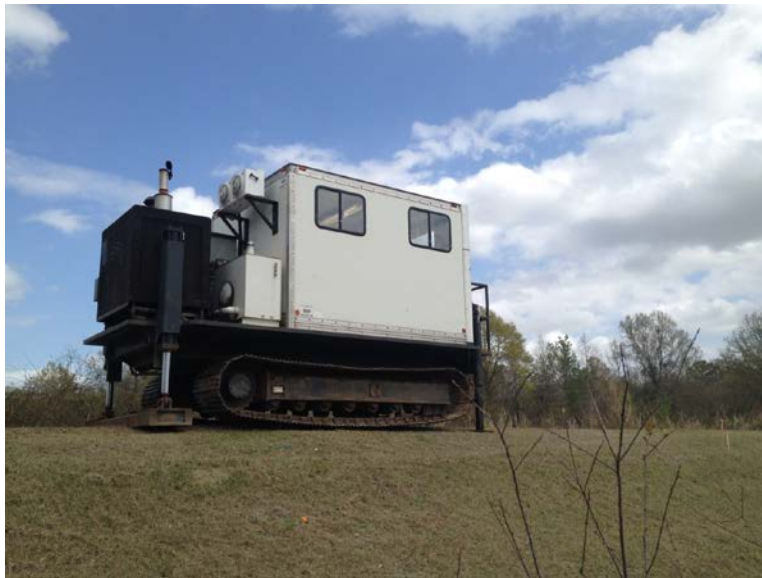
Photo 1. Track mounted CPT rig.
