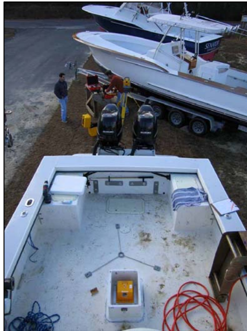
Figure 5. Photo of the centerline and instrument survey by NGS.
